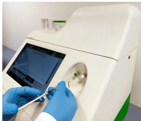
Injecting Opti-Count® reference material particles into a LUMiSpoc® for method validation. ©LUM GmbH
