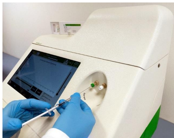
Figure 1: Injecting Opti-Count® reference material particles into a LUMiSpoc® for method validation. ©LUM GmbH
